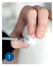
The valve dummy requires a flat support surface and must be firmly screwed in place.
