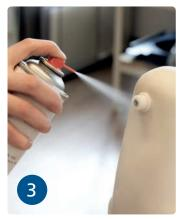
The model and dummy must be insulated to facilitate demoulding.
