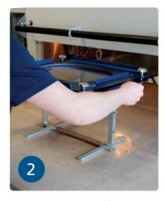
Prepare the thermoforming material and heat to processing temperature.
