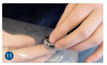
Insert the valve from the inside and screw it on from the outside. There must be a sealing ring between the socket and the valve.
