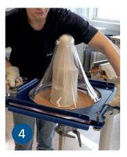
Deep-draw the heated material over the plaster model and dummy.
